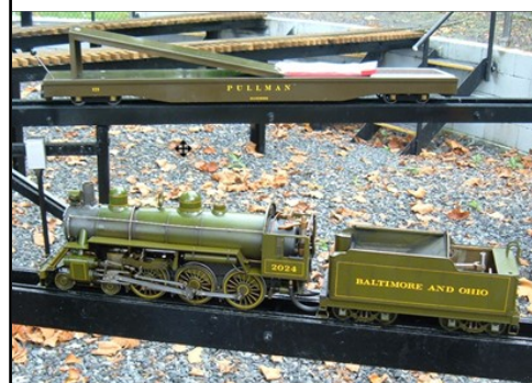
While the loco is 2.5" gauge, the lay-down driver's car was 4.75" and had to be separated at the steaming bays since the 2.5" steaming bay does not accommodate 4.75" gauge. Even though the loco was in 'clean up mode' (no cab roof or pump cover), Bob made sure to roll her so that the side rods would appear down in the classic 'steam loco' photo position.
