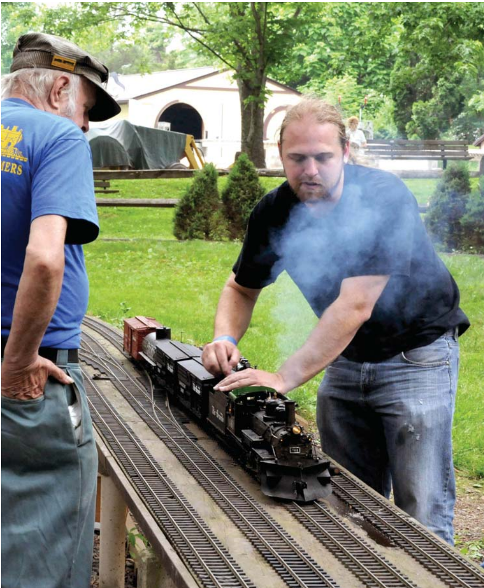
Justin Koch’s coal-fired narrow gauge K27 started life as an Accucraft electric model. Justin converted the engine to coal-fired steam.
