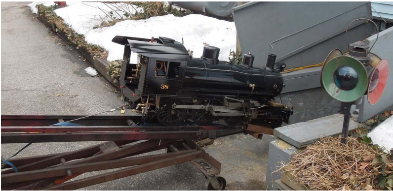
L-R from Top: Locomotive on temporary track lifted up onto the top step of basement stairs by hand; Looking down the steps at locomotive before winching it up; Temporary track attached to the dolly lift and loco being winched up; Winch attached to my truck hitch powered by a heavy duty battery charger; Loco was loaded into the truck to be transported to the garage; The loco was then transferred to the test dolly.
