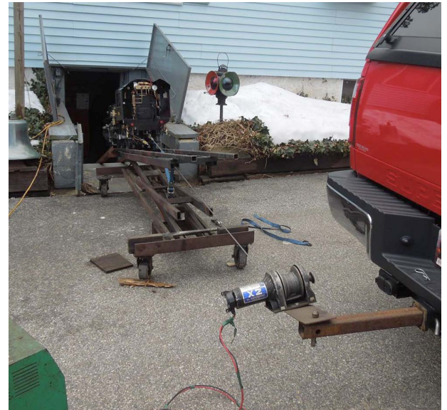
L-R from Top: Locomotive on temporary track lifted up onto the top step of basement stairs by hand; Looking down the steps at locomotive before winching it up; Temporary track attached to the dolly lift and loco being winched up; Winch attached to my truck hitch powered by a heavy duty battery charger; Loco was loaded into the truck to be transported to the garage; The loco was then transferred to the test dolly.
