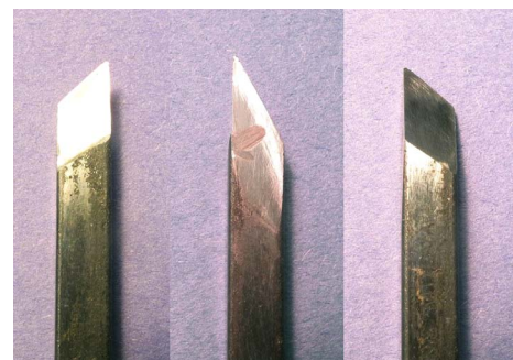
Fig.2. An LBSC dual-function lathe tool, showing ground and stoned surfaces on left side, top and right side.
